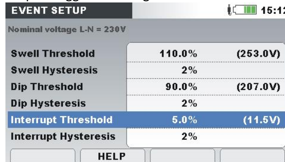
Figure 5.24: Waveform recorder setup for triggering on voltage events
