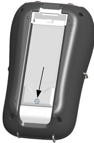
Figure 7.2: Closing the battery compartment cover
